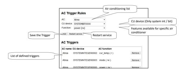
AC Trigger Rules used to pair the CU element and AC function. This way you can store AC states to CU and control AC from CU.
