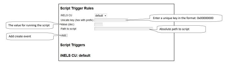
LeventScript uses ASCII protocol, which must be turned on in IDM program, into a free port and in bookmark Configuration in iMM CC insert ASCII port for communication.
