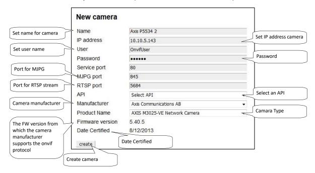
1 The service port is the ONVIF port usually set on port 80. If the camera is behind NAT it is necessary to redirect to the router and this port otherwise the camera cannot be configured
